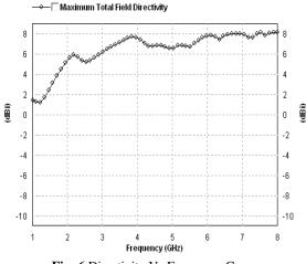
Fig: 6 Directivity Vs Frequency Curve
