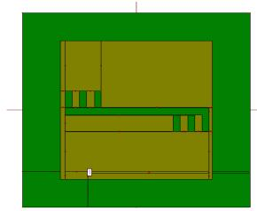
**Fig: 2.** Microstrip Patch Antenna with back to back E shape slots Feed at (-7.57, -13.35).
