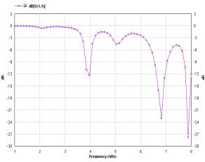
Fig: 3. Return loss Vs Frequency Curve of Microstrip Patch Antenna with back to back E Shape Slots Antenna
