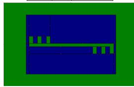
Fig: 1. Back-to-back E Shaped Patch Antenna
