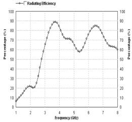
Fig: 8. Radiation Efficiency Vs Frequency Curve
