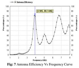
Analyzing the efficiency curve shown in figure (7) it can be clearly observed that the designed antenna structure provides an antenna efficiency of 80%. Further radiation efficiency of the antenna structure is shown in figure (8).
