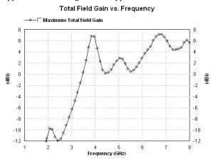
**Fig: 5.** Total Field Gain Vs Frequency Curve Another important parameter related to the antenna gain is antenna directivity which is shown in figure (6)
